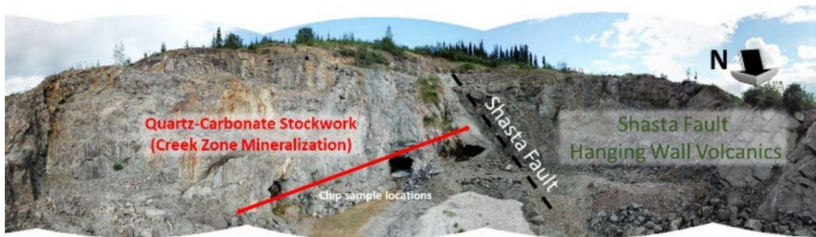
Figure 9-32: Chip Sample Location at Creek Zone Pit on SW pit wall
