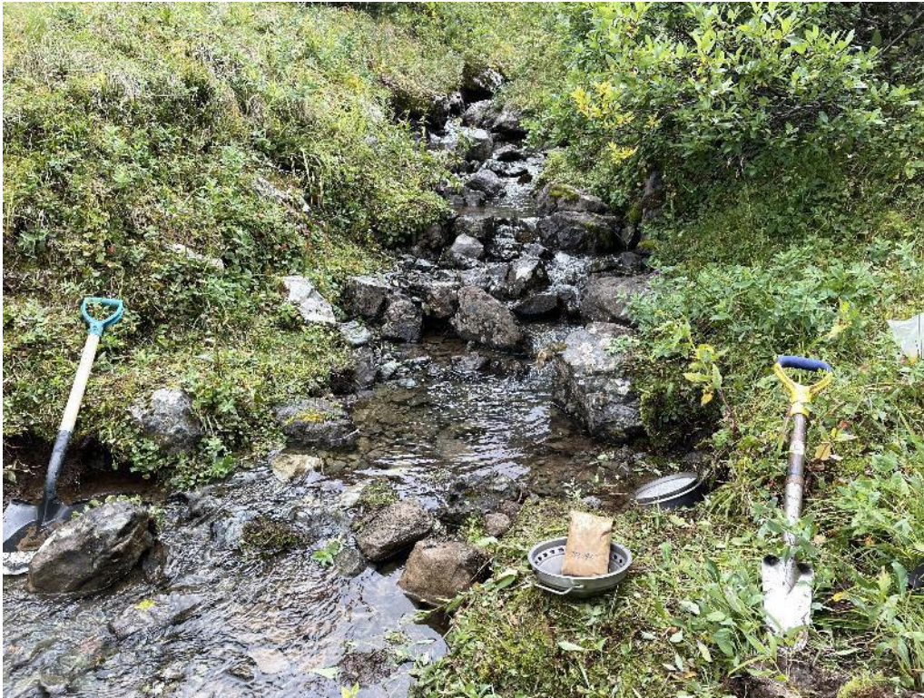
Figure 9-53: Example of a 'Wet' LDS Site and Completed Sample
