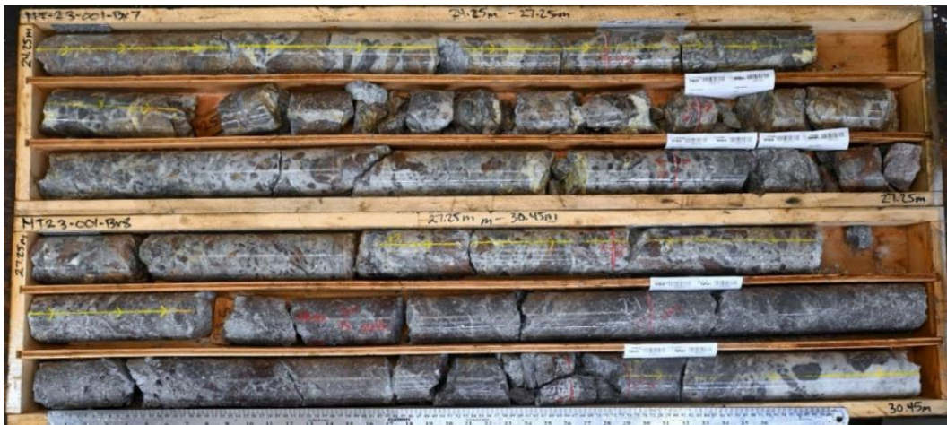
Figure 9-78: Drill core photo of MT23-001 which graded 21.30 g/t Au over 7.0 m at 24.0 m depth
