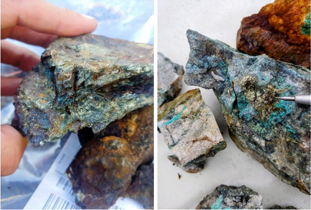
Figure 4 – Rock Samples Taken at the Erebus Target Area (Left: Sample G676066, Mafic Volcanic disseminates with chalcocopyrite/pyrite with 11 % Cu in Float directly below inaccessible Cliff; Right: Sample D00209783 Quartz Monzonite with disseminated chalcocopyrite/pyrite, malachite/azurite on fracture surface and pervasive potassic alteration with Mo veining grading 0.45 % Cu & 32.4 ppm Mo in outcrop).
