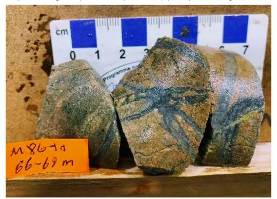
**Figure 3** – BK86-10 from 66.0-66.07 m. Strong potassic altered dacite with multi-generational quartz/quartz carbonate and epidote veining.
