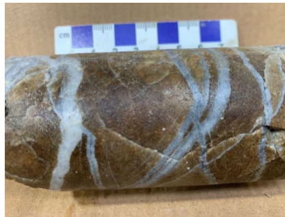
Figure 3. 97.0 m. Intensely potassic and sericite altered dacite containing multiple generations of quartz veins hosting sulphide minerals (disseminated pyrite with minor bornite, chalcopyrite, molybdenite and sphalerite).
