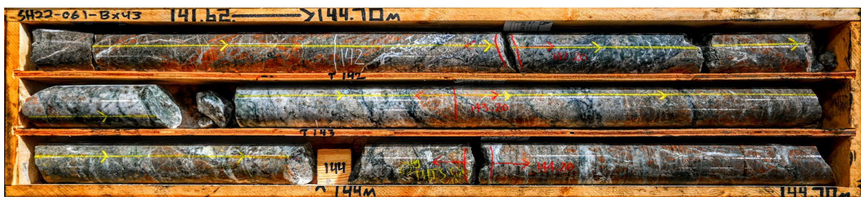
Image 1. Shasta drillhole SH22-061 from 141.62-144.70 m; sample, 143.2-145.2 m (downhole) grading 12.72 g/t Au and 422 g/t Ag [18.00 g/t AuEq 1 ].
