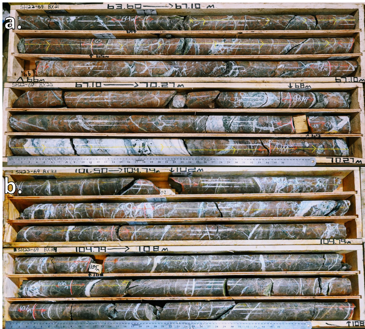
Image 2. SH22-069; an example of intense quartz-carbonate veining and/or hydrothermal breccia comprised of a quartz, carbonate and chlorite matrix, pervasively silica altered, with angular to sub angular potassic altered clasts, intersected a. 63.6 – 70.3 m b. 101.5-108.0 m
