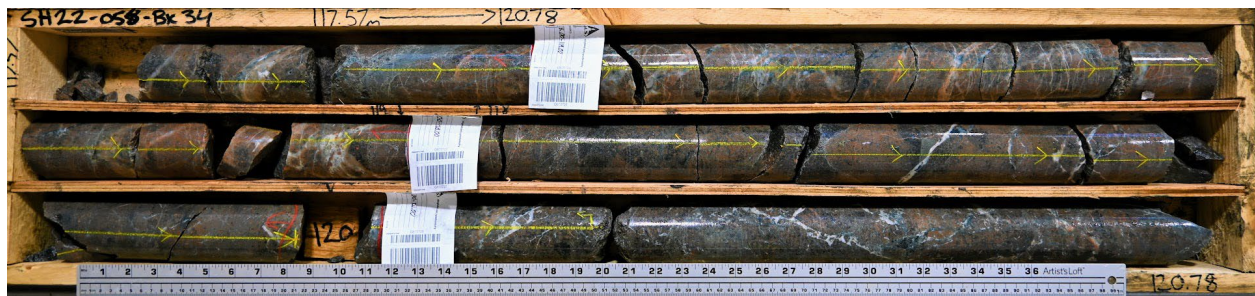
Image 3 – SH22-058 (117.6 – 120.8 m). Vein/brecciated Potassic altered, silicious volcaniclastic rocks hosting pyrite, acanthite sulphides.
