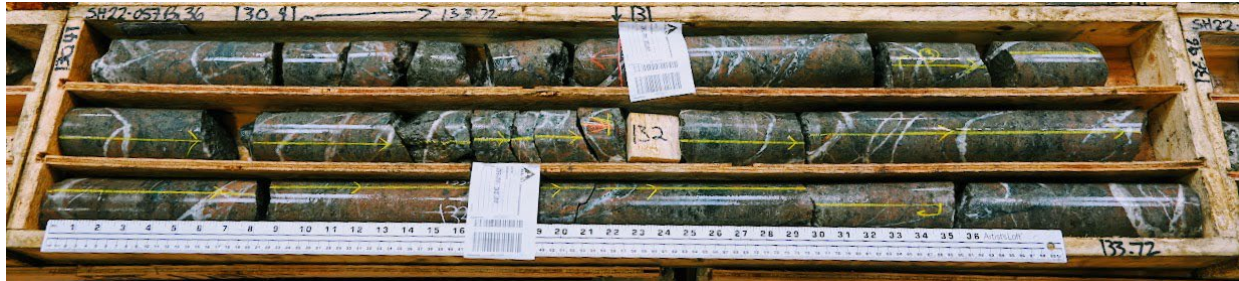
Image 2 – SH22-057 (130.41 – 133.7 m). Vein/brecciated Potassic altered, silicious volcaniclastic rocks hosting pyrite, acanthite sulphides.
