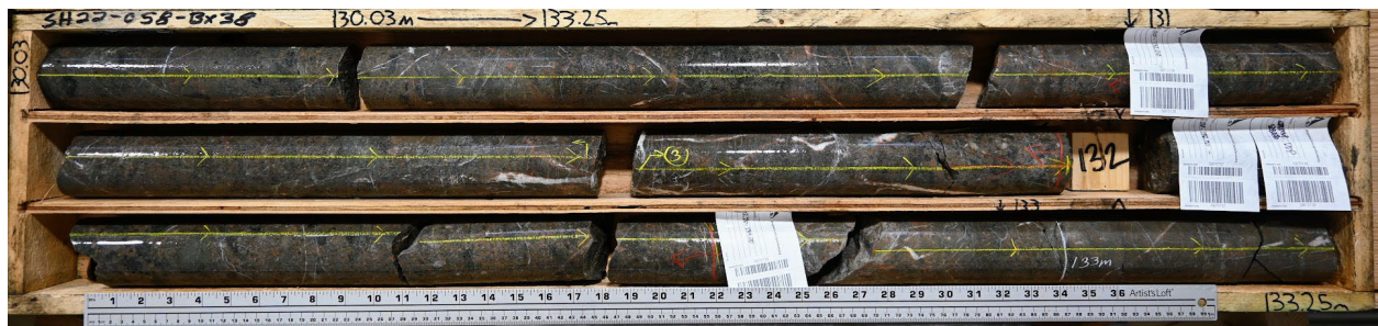
Image 4 – SH22-058 (130.0 – 133.3 m). Vein/brecciated Potassic altered, silicious volcaniclastic rocks hosting pyrite, acanthite sulphides.
