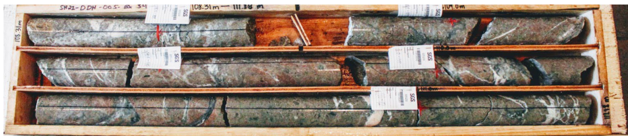
Image 1 – SH21-005 (108.3 – 111.4 m). From 108.5 to 111.0 (2.5 m) 1.62 g/t Au, 73 g/t Ag, 2.53 g/t AuEQ. Vein/brecciated Potassic altered, silicious volcaniclastic rocks hosting pyrite, acanthite sulphides.
