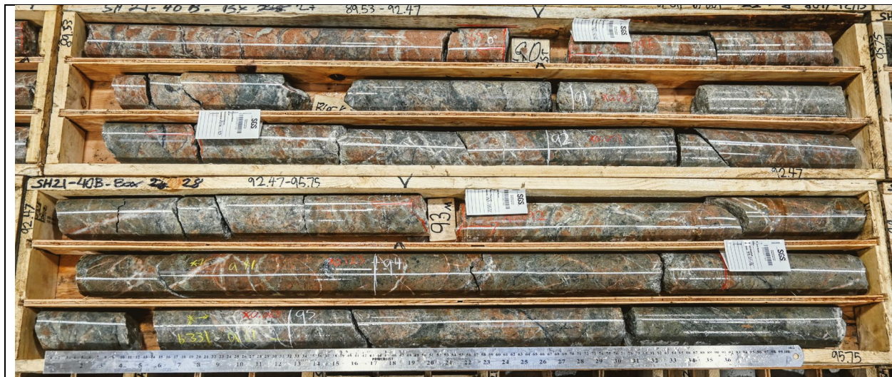
Photo 1. Mineralization encountered in drillhole SH21-040B from 89.53 – 95.75 m; calculated composite (absolute, no cut off) through 88.5 to 93.0 m (4.5m) 13.22 g/t Au and 34 g/t Ag [13.66 g/t AuEq*] .
