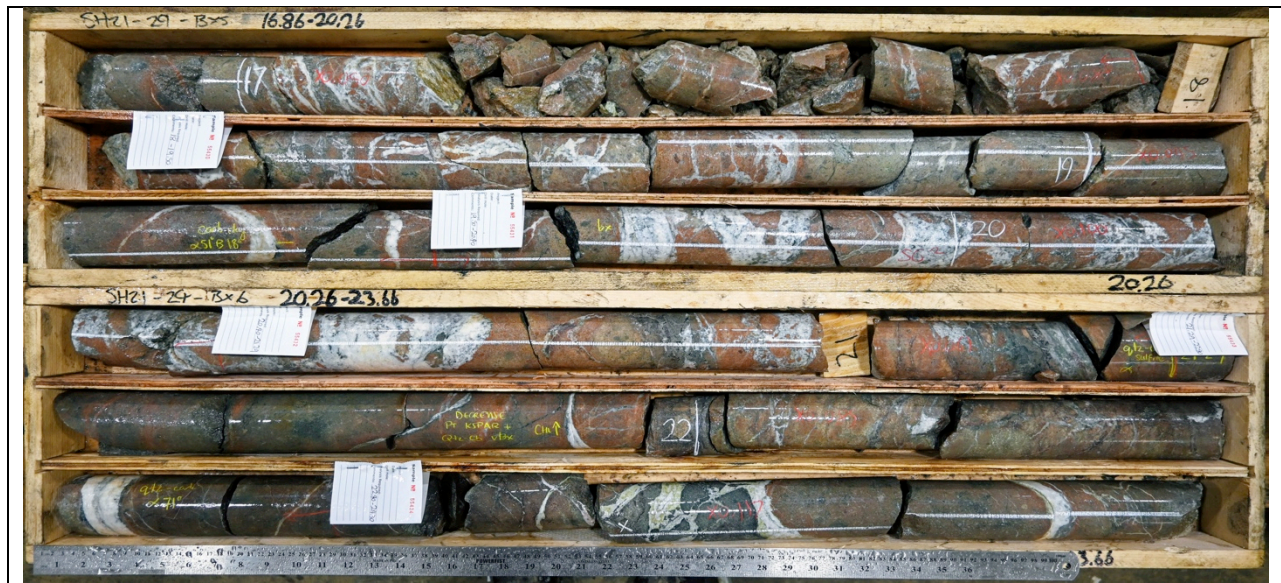
Photo 1. Mineralization encountered in drillhole SH21-029 from 16.86 – 23.66 m; calculated composite (absolute, no cut off) through 19.5 to 22.8 m (3.3 m) of 4.89 g/t Au, 326 g/t Ag [8.97 g/t AuEq*] .
