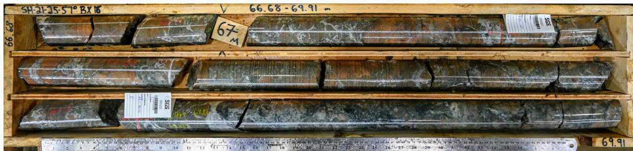
Image 1. Shasta drillhole SH21-025; mineralization encountered grading 5.61 g/t Au and 196 g/t Ag over 1.5 m from 67.5 m to 69.0 m depth.
