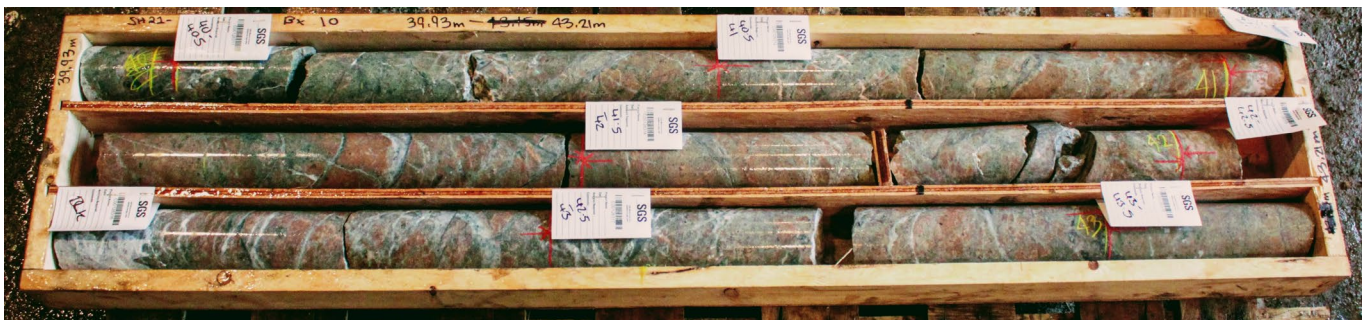
Figure 2. Shasta drillhole SH21-006; mineralization encountered grading 1.46 Au g/t, 69 g/t Ag [2.32 g/t AuEq*] from 43.5 m to 46.5 m depth.
