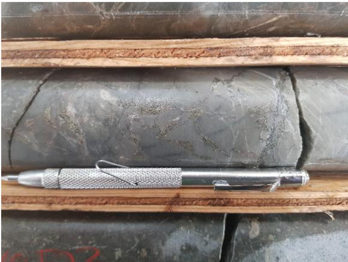
Image 2. Drill Hole OP21-002 detailed photo of 358.75 m pyrite replacement in quartz veining.
