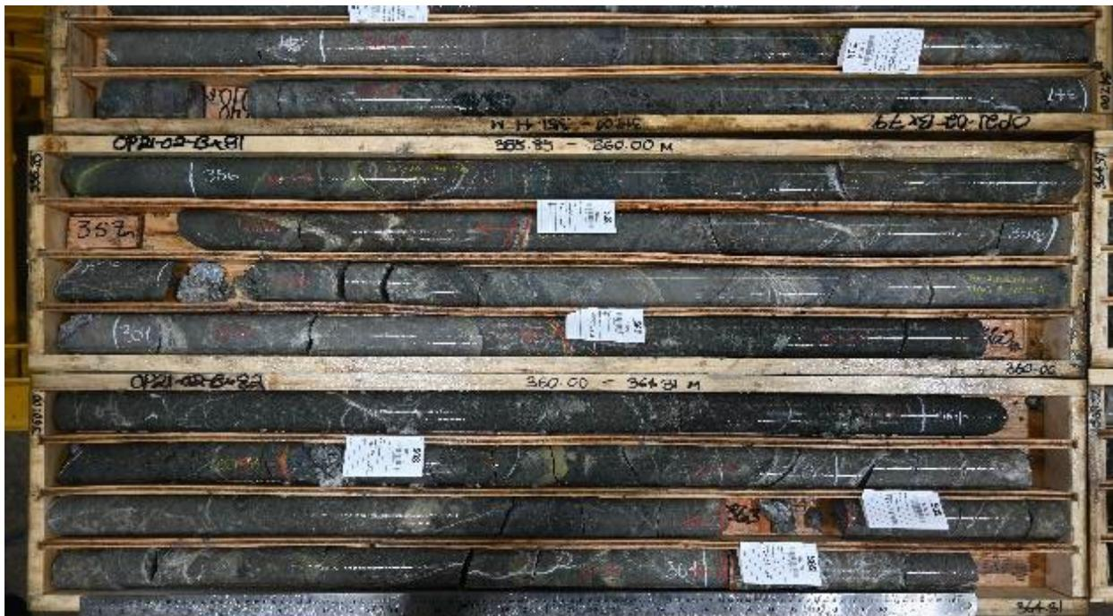
Image 1. Drill Hole OP21-002 from 355.85-364.31 m - banded, ash tuff, intense silicification, brecciated by quartz veining with up to 5 % disseminated pyrite and an additional 5 % pyrite replacing quartz-carbonate veins.
