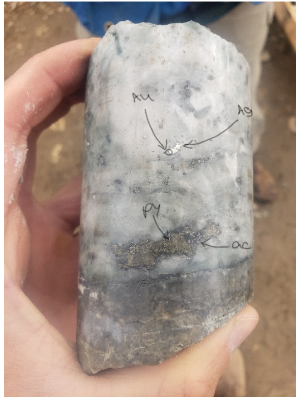
Picture 1. Shasta drillhole SH21-004 at 69.9 m depth quartz-carbonate vein with acanthite, pyrite and native silver.
