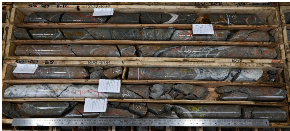
Figure 4. Core photo showing silicified potassic-altered volcanoclastics with quartz vein stockwork (intersected between 57.2 - 63.6 m in hole SH21-027).
