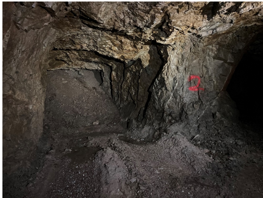
Figure 1: “Pillar 2” of the 1300 level at Shasta Mine. Grab sample 3693868 was taken from vein and stockwork material visible in this image.
